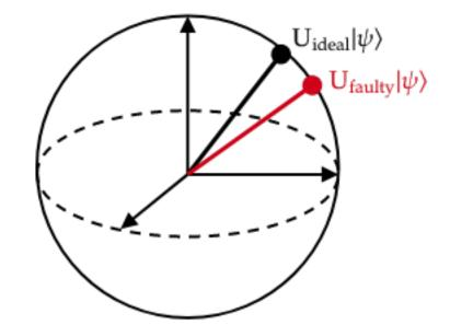
Need smaller gate noise to perform quantum error correction
